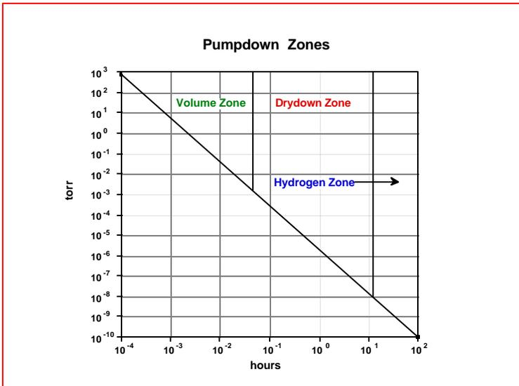
*A pumpdown curve from air shows the three major zone divisions based on residual gases: the volume zone dominated by air, the drydown zone dominated by desorbing water vapor, and the hydrogen zone dominated by hydrogen.*
