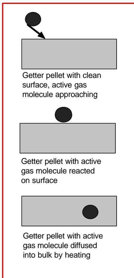
*Getter pellets can react with gas molecules, which usually form a low vapor pressure ceramic compound.*
