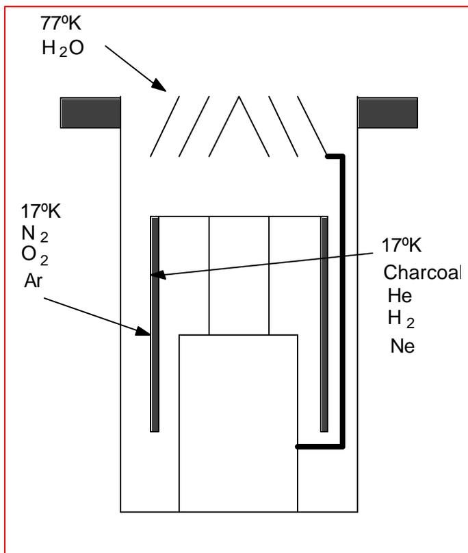
*The various cold arrays within the cryopump body show their specific pumping capability. The chevrons in the pump inlet are positioned to pump the main gas load in most systems, water vapor. Other gases pass through the water pumping array, and are then pumped according to their degree of possible condensation.*
