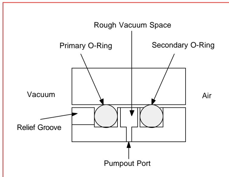
*The relief groove allows trapped volumes of gas to be pumped out of the O-ring groove and the rough vacuum space with pumpout reduces the primary O-ring's permeation rate. Source: Phil Danielson*
