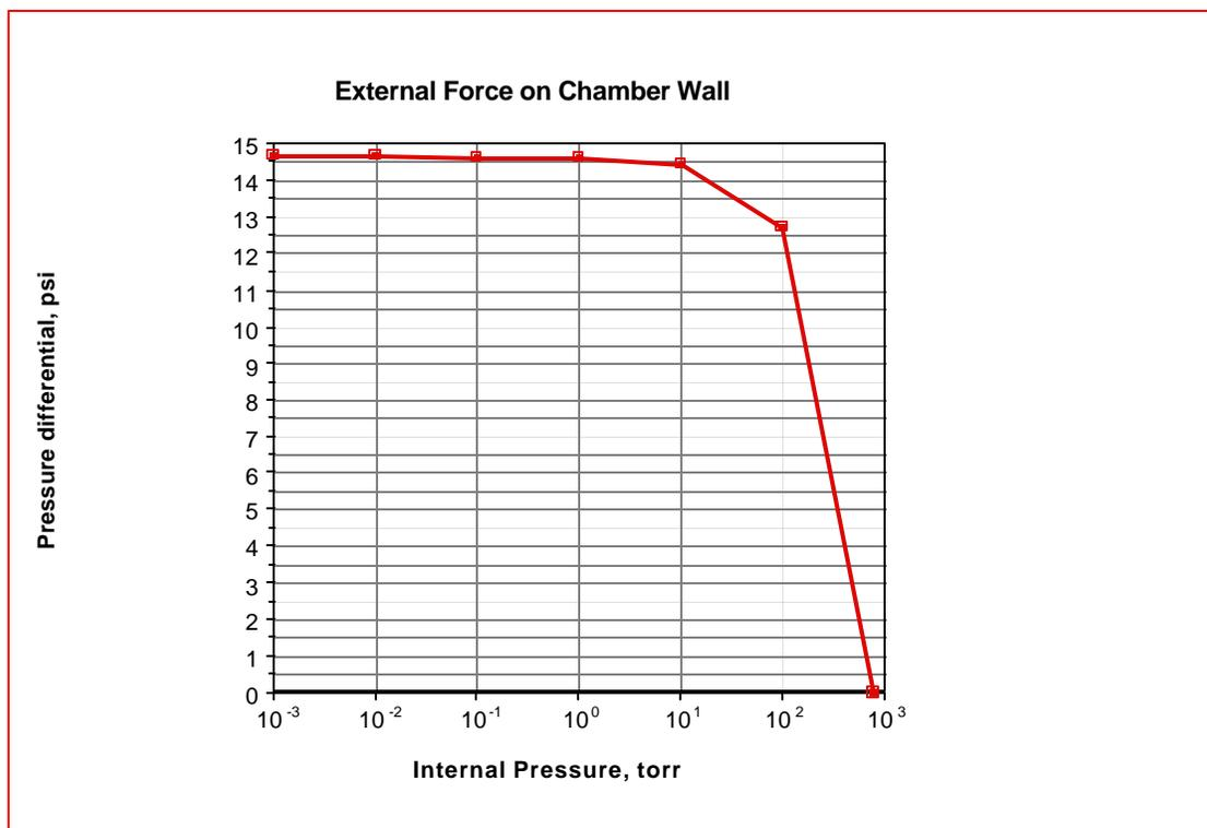
*As the pressure within the vacuum chamber is reduced, the ambient pressure increases the force on the chamber wall, but the increase in force is negligible below a few torr.*
