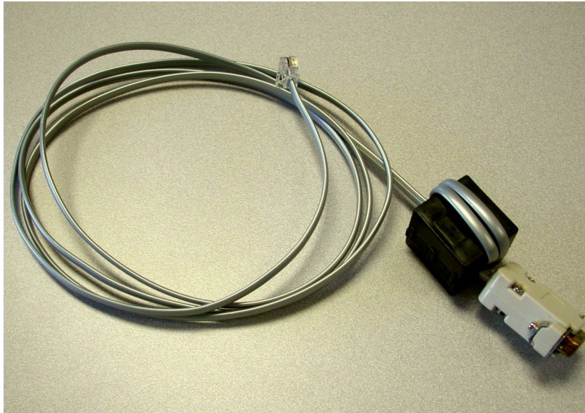
Figure 4: I/O Communication Cable for Remote Connections
